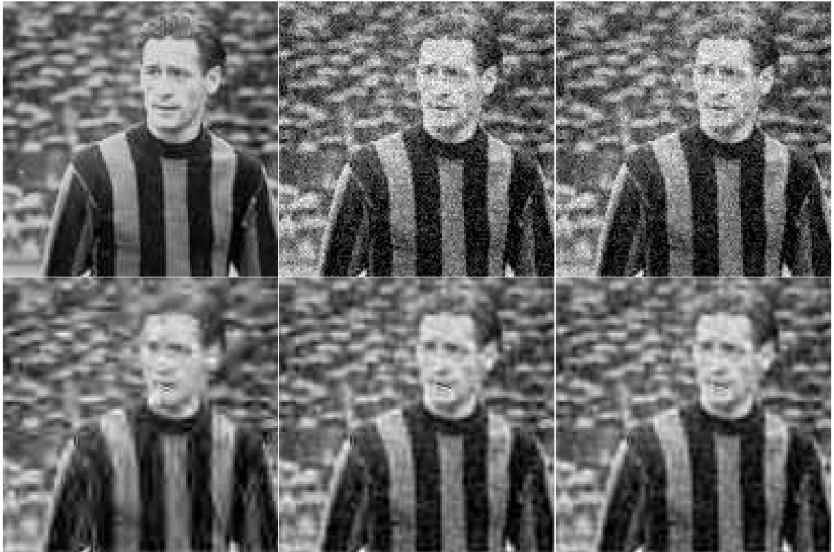
Figure 2: The MDL denoising methods in action. Top row (from left) Original (size 128 \times 128 ); noisy (noise std.dev. 20.0); original MDL denoising [21]. Bottom row : Left to right, gradual improvements of the MDL denoising method [22].
