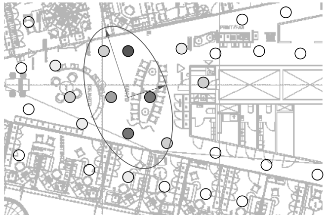
Figure 2: Uncertainty ellipse. Probabilities at a discrete set of locations are denoted by circles; dark shading implies high probability. The ellipse centered at the expected location has axes parallel to eigenvectors of the variance-covariance matrix and lengths proportional to eigenvalues.
